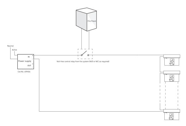
Note: Max. cable length over entire loop when using shielded twisted pair cable is 500 m.
